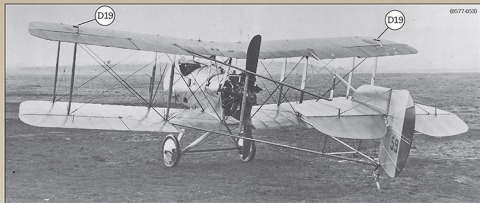
AMC DH.2 5938 is from the same initial production order as Lanoe Hawker's 24 Squadron 5964 and is seen here in factory fresh condition. Note the spring type aileron control horn returns, 2 blade propeller, single pitot tube and lack of a compass and fairing.
