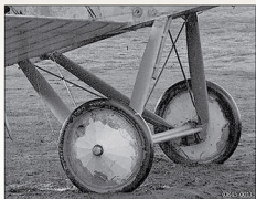
^ > Undercarriage detail from DH.2 5938 as seen on page 13. Note the grey painted struts and black rubber tyres.
